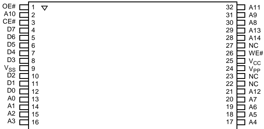
32-Pin TSOP—Reverse Pinout
